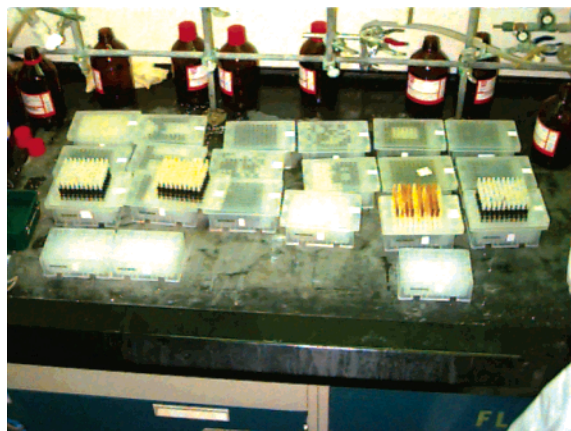
Figure 12. Cleaving samples from crowns mounted on pin racks directly into 96-well plates.
