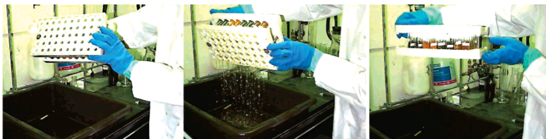
Figure 7. Filtering 40 reaction vessels in parallel with the Wheaton Sandwich.
