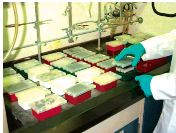
Figure 11. Washing crowns in the pin rack format.
