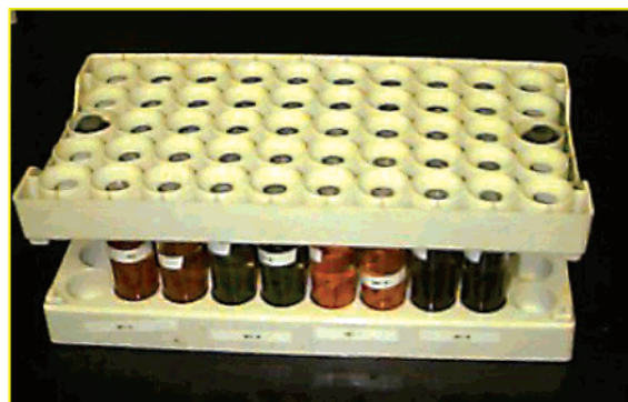
Figure 6. An 8 × 5 array of 40-mL vials in the Wheaton Sandwich.
